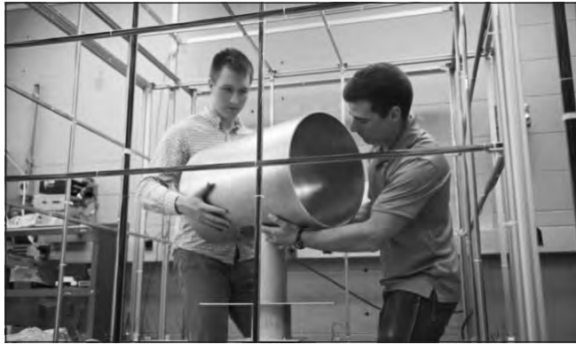
Conducting an experiment they devised to facilitate capture and disposal of orbiting space junk, Nicholas James (right) and co-researcher James Figura position a cylinder, representing a rocket body, inside the MIT Space Systems Lab's Helmholtz cage. The cage will generate magnetic fields that will both rotate the cylinder and then force it to stop rotating, enabling capture. Photo by William Litant.
